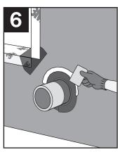
Detail penetrations by wrapping 3M™ Ultra Conformable Flashing Tape 3015UC around the penetration, ensuring the lap ends at the bottom with a minimum of a 2" overlap. The negative lap of this detail will be covered when the field membrane is installed. Apply 3M 740UV, or similar compatible sealant along top half of tape edge and tool smooth.
