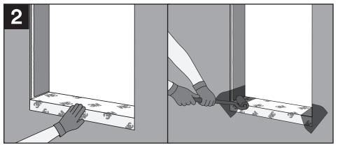
If 3M™ Air and Vapor Barrier3015NP or 3015TWF will be used as the sill flashing tape, first cut it the width of the window and apply over the sill extending at least 2" onto the wall. Then apply 3M™ Ultra Conformable Flashing Tape 3015UC in the corners, extending over the sill tape and up the vertical side of the frame ensuring a minimum 2" overlap in all directions. Apply pressure with a J-roller.
