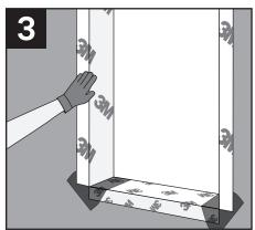
To detail the vertical sides of window, cut 3M™ Air and Vapor Barrier 3015NP or 3015TWF the same length as the height of the frame. Extend onto the wall and overlap the sill flashing a minimum of 2" to prevent negative laps.
