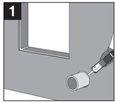
Prep window opening and penetrations. Caulk gaps and ensure all mortar joints are tooled or struck flush. Gaps wider than 1/2" must be filled with backer rod and caulk prior to applying 3M™ Ultra Conformable Flashing Tape 3015UC.
