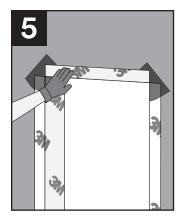
To complete the window detailing, cut a piece of 3M™ Air and Vapor Barrier 3015NP or 3015TWF the same width as the window. Overlap a minimum of 2" onto the wall and over the 3M™ Ultra Conformable Flashing Tape 3015UC in the upper corners.
