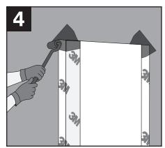
Apply 3M™ Ultra Conformable Flashing Tape 3015UC in the corners, extending over the vertical sides of window flashing and directly to the wall. Ensure tape is applied with a 2" minimum overlap in all directions.
